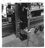
Oxyfuel torch including hoses, solenoid valves on magnetic quick change system. Uses the same motorized station and lifter as the plasma torch. Allows the operator to quickly switch between oxyfuel and plasma cutting.
