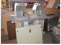
#34 • INDUSTRIAL BUFFER STATION DIXON (MODEL #29) DUAL-WHEEL BUFFER WITH DUST COLLECTION SYSTEM. NOT TESTED.
